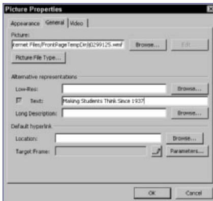
Figure 232-2: The Alternative Representations section allows you to type text to describe a graphic within your Web page
