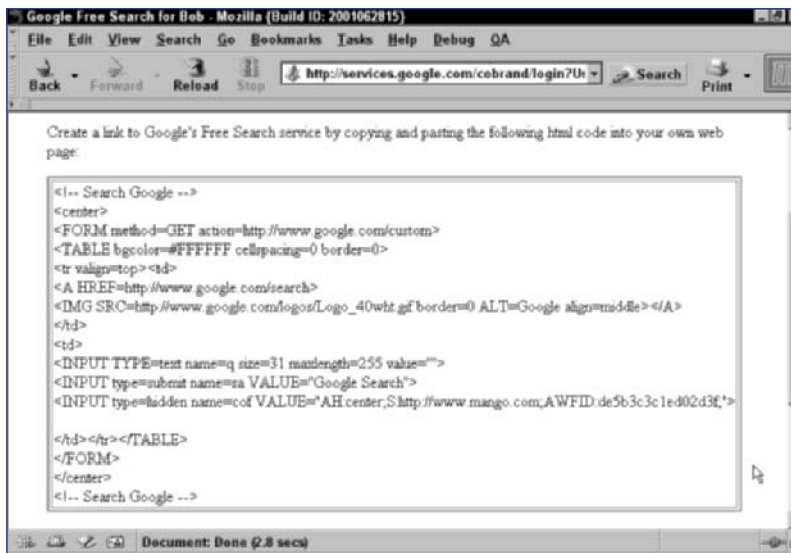
Figure 110-2: The source code Google provides for you to copy and paste into a document on your Web site
