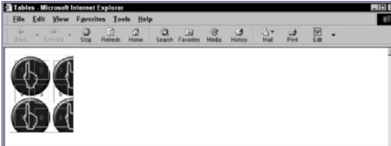
Figure 48-2: Background images tile from left to right and top to bottom across the element they're applied to.
