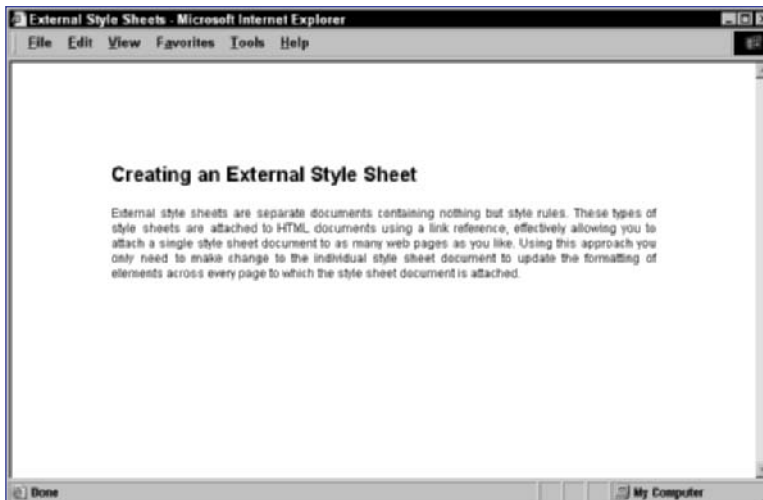
Figure 75-2: An HTML page whose formatting is defined solely in an external style sheet
