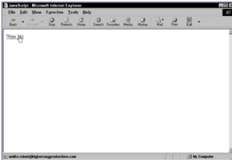
Figure 106-1: The mailto: link is written with the “Write Me” text specified in the document.write statement, and when it’s moused over, the completed link is referenced in the status bar.
