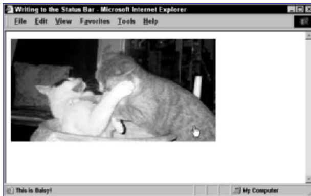
Figure 105-2. Changing the status bar with an onMouseOver event so that it reads "This is Daisy!" when the picture is moused over
