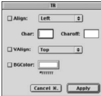
Figure 143-2: Setting attribute values for the <tr> tag in the TR dialog box
